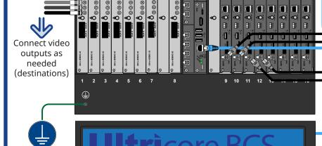
Note: Terminate the REF LOOP connector and set the DIP to TERM if the router is the last device in the reference chain.
